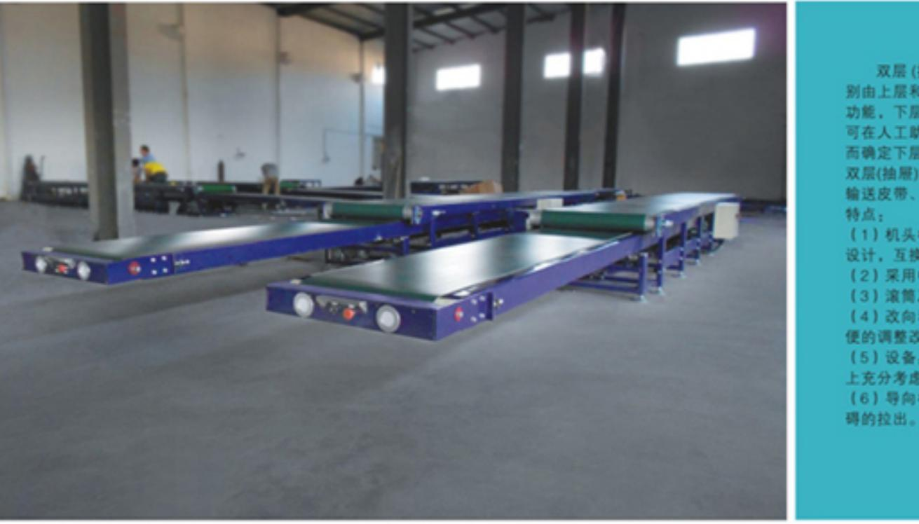
Lapped Drawer Belt Conveyor applied in rapid delivery and loading goods. It includes two belt conveyors which is lapped, upper belt conveyor for conveying articles when the Lower layers of belt conveyor for loading. Lower layers of belt conveyor can be extendable or retractable freely. In structure, it contains drive motor, Tensioning unit, Belt, Framework, Turnabout unit, Guide unit, Electric control box. Features as following:
