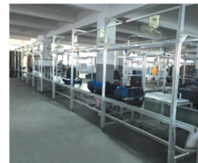
工装流水线 Gravity roller and steel ball line
