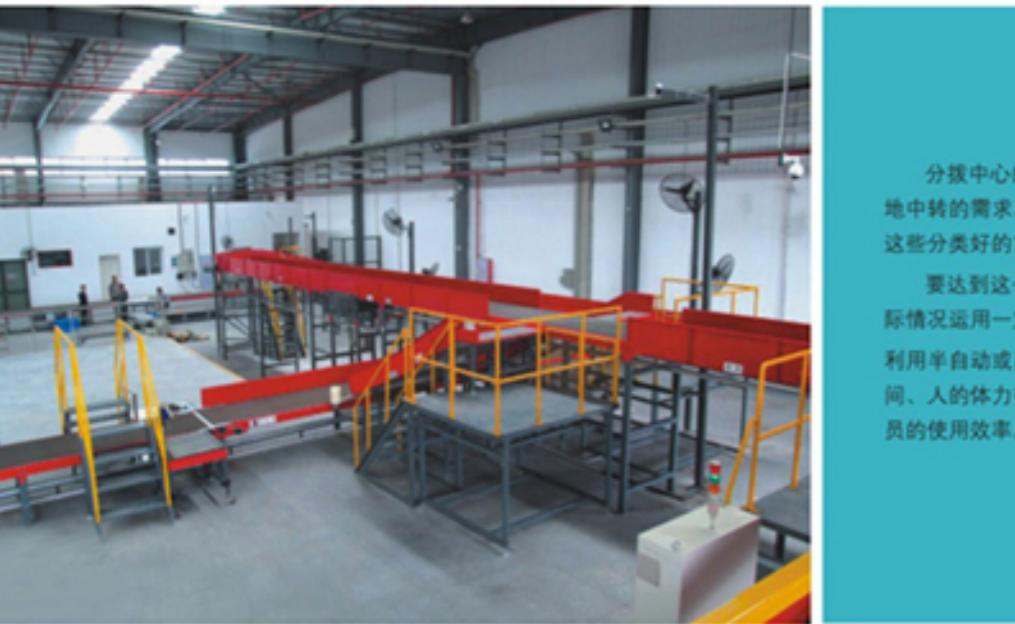
Distribution center requires rational planning and efficient sorting to meet the needs of transit, must unload and classify goods by location in the shortest time, and send the goods to the designated place and quickly loading to distribution.
