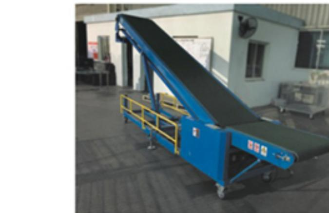
•铝合金倾斜皮带机 Inclining Belt Conveyor in Aluminum
