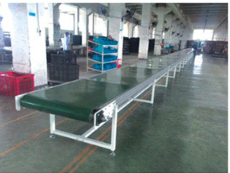
铝合金皮带输送机 Belt Conveyors in Aluminum frames
